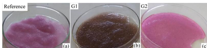
**Figure 2.** Adhesion test for glass beads: (a) Reference glass bead with no adhesion coating treatment, (b) Glass bead G1; (c) Glass bead G2
